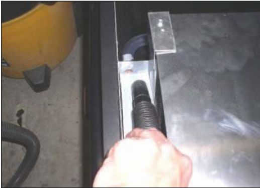
Figure E: Clean Drain Opening & Drain Pan
