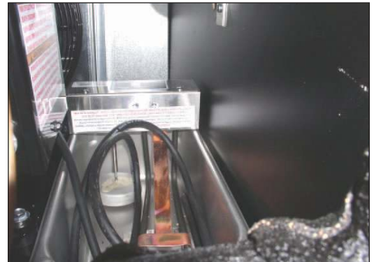
Figure B: Dissipater Heater & Float
