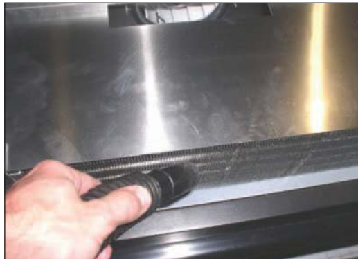
Figure D: Clean Coil with a Wet/Dry Vacuum & Brush
